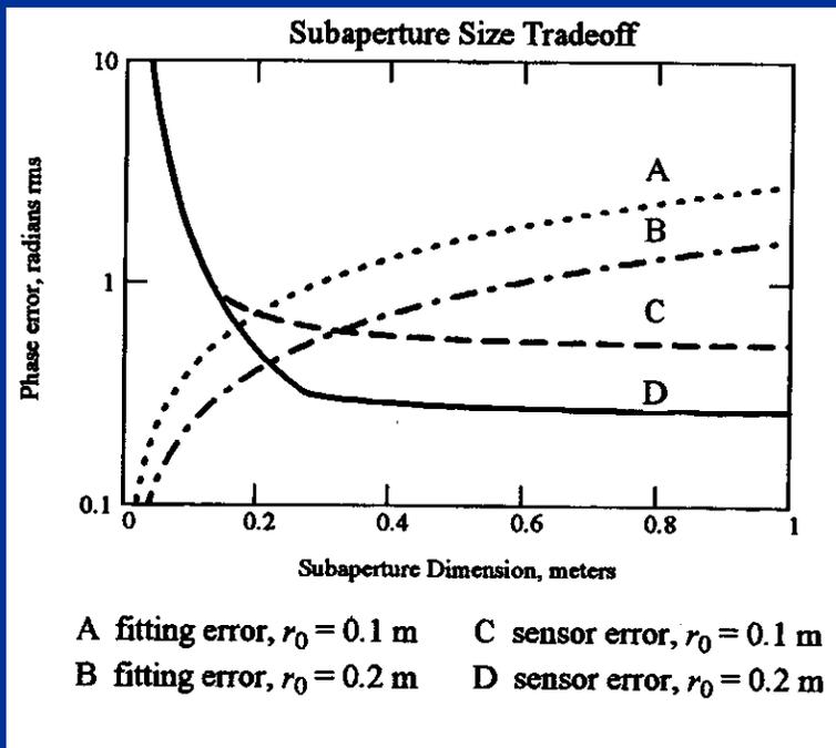
$$\sigma_{\phi}^2 = \left[ 3.5\theta_b \frac{d}{\lambda} \right]^2 \frac{R^2 n_{pix}}{(Flux \times T_{int})^2} + \mu \left( \frac{d}{r_0} \right)^{5/3}$$
